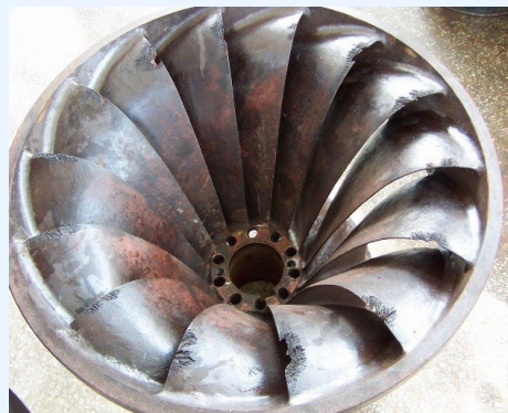
WORN TURBINE REPAIR /GOLD 627
