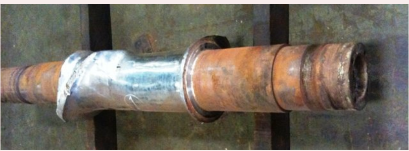
Wear on Rubber Kneader (mixer) GOLD 330 For rebuilding and protection
