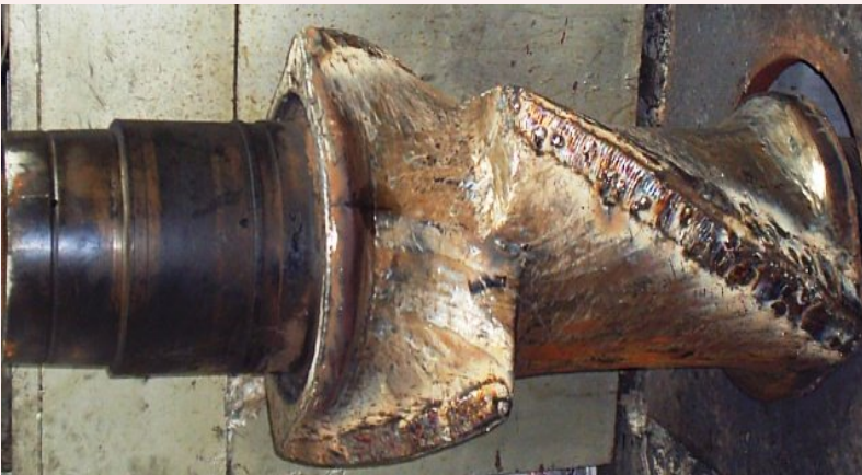
Rubber Mixer / GOLD 330- for restoring HB 50 C0 or long term protection/ hardfacing
