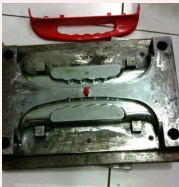
Damages on plastic mold. Repair with 330 T or 728 T (GTAW)
