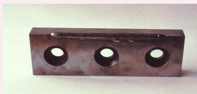
Damage and wear on cutting knives: Repair with ARCWEL 330 T /7201 T
