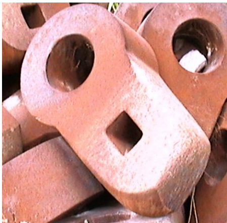
REBUILD WORN CRUSHERHAMMER
