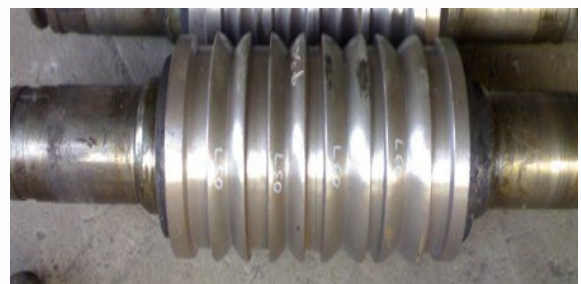
REPAIR AND REBUILD WORN ROLLER
