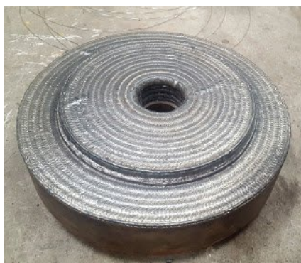
BALL VALVE : HARDFACING WITH 1047 T
