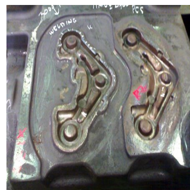
FORGING DIE: REPAIR WITH 1049 T
