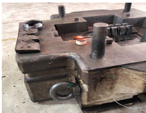
ALUMINIUM DIE CAST MOLD REPAIR WITH GOLD 728 /1015 T
