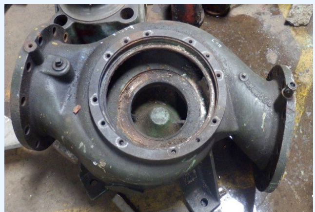
PUMP HOUSING REPAIR/PROTECTION
