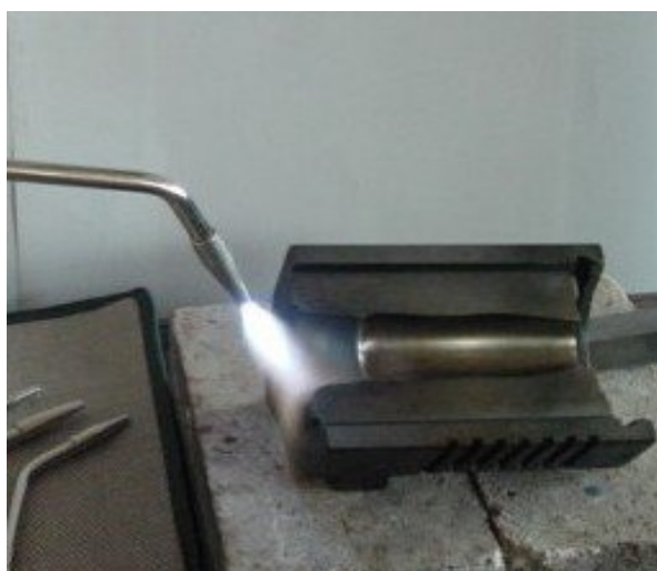
GLASS MOULD REPAIR ARCWEL 2020 SF
