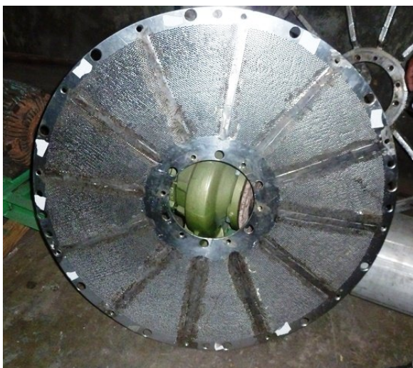
STAINLESS STEEL SCREEN –REPAIR ARCWEL 22 B SN/AG SOLDER
