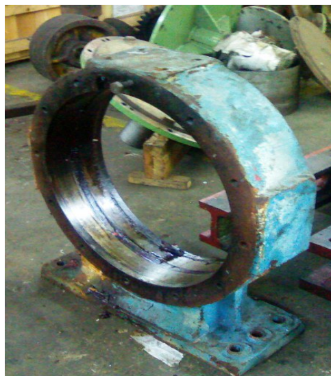
WORN BEARING HOUSING : E- 190/ BABBITT 90 AS
