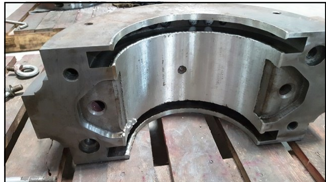
BEARING HOUSING REPAIR with ARCWEL BABBITT 90 SN –AS
