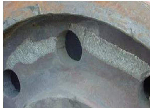
Kiln tire repair weld
